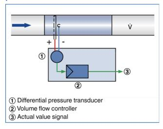
Differential pressure sensor for the measurement of non-contaminated supply air.
