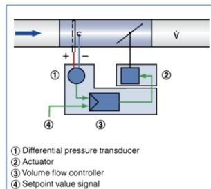
**Universal controller, static, for VAV terminal units, volume flow control**
